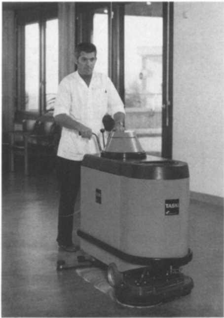
Fig. 6. Industrial sweeper truck using gelled-electrolyte traction cells.
